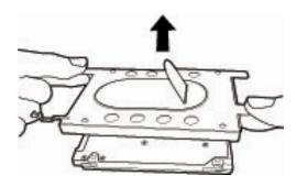
Figure 4-6 Separating the HDD and HDD holder
